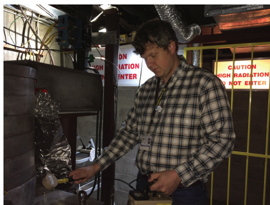
CAMD radiation safety officer Charles A. Wilson IV verifies shielding on a Klystron at the LSU J. Bennett Johnston Sr. Center for Advanced Microstructures and Devices.
